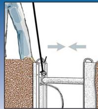
Release the shoring fluid at fitting using the release tool.
