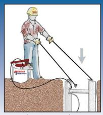
Lower shore into trench per O.S.H.A. requirements. Use release tool nearest to you and removal hook on far side.
