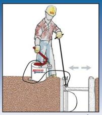
Pump to minimum pressure of 750 psi. Disconnect hose from fitting using the release tool.
