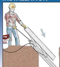
Connect hydraulic hose line to fitting. Position shore at edge of trench.
