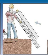
Complete hydraulic shore assembly folds flat for portability to next location. Always keep fingers clear of pivot pump.
