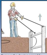
Remove the shoring assembly from trench using both release and removal hook.
