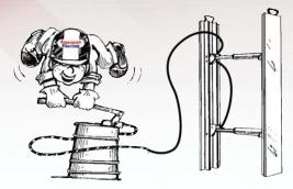
Pump with gauge, valve, hose and quick disconnect fittings. Pump's gauge regulated pressure ensures evenly applied loads. Wire braided hoses are protected by spring guards.
